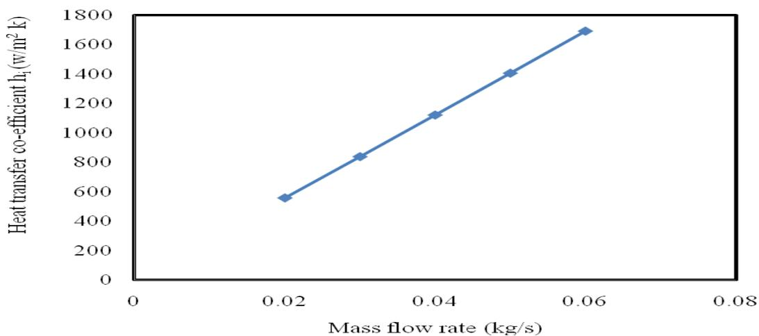
Figure 1: Variation of Heat transfer coefficient on different Mass flow rate at constant temperature
