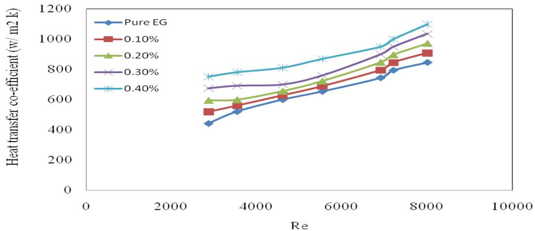
Figure 4: Variation of heat transfer co-efficient on reynolds number
