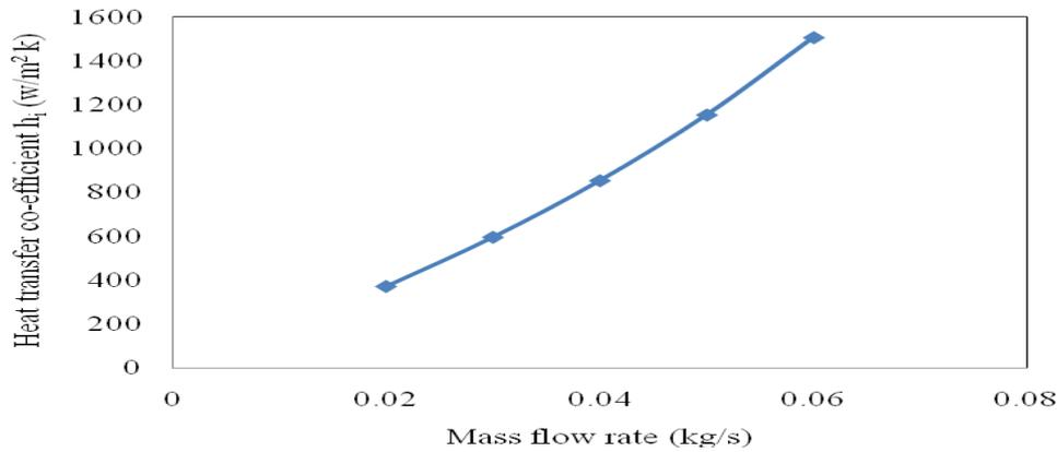
Figure 2: Variation of Heat transfer coefficient on different Mass flow rate
