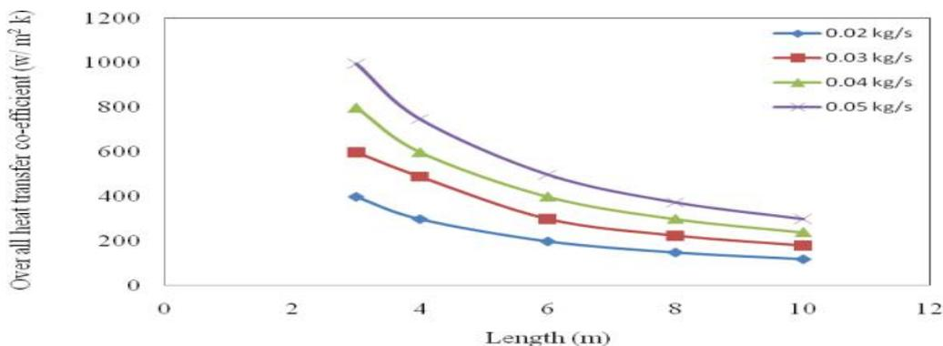
Figure 3: Variation of overall heat transfer co-efficient over different pipe length
